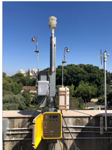
Nephelometer, filter station and meteorological station in Rehovot
